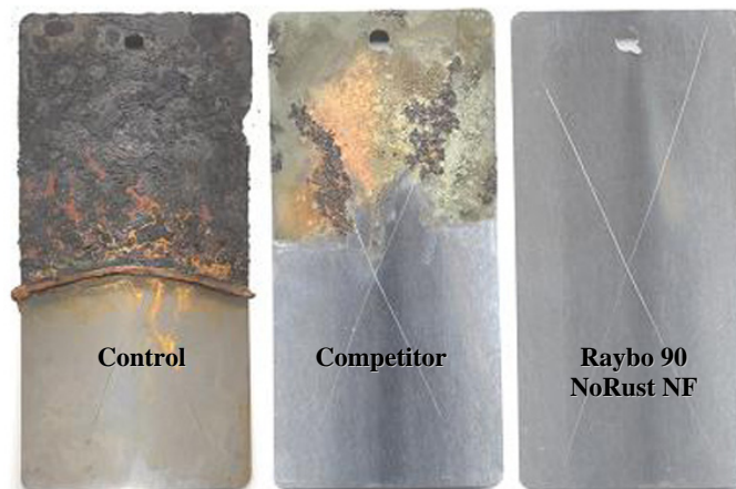
Panels partially immersed in UCAR 379 for 23 days (120°F, pH adjusted to 8.3)
